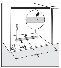
Position the fitting bracket on the center line. Use the mark on the bracket as a guide.
